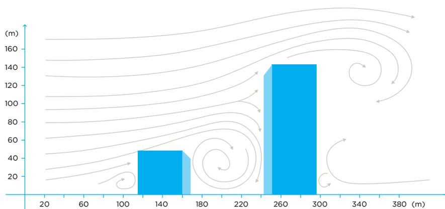
The principal flow patterns in two dimensions when wind passes over buildings of different heights. When more buildings are involved, as in normal urban areas, it becomes impossible to accurately predict the flow without experiments or numerical simulations.
